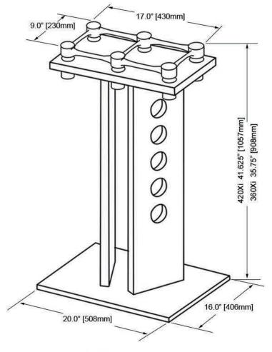
up to 100 lb. effective capacity inserts provide up to 6.5 degrees of tilt upward or downward
